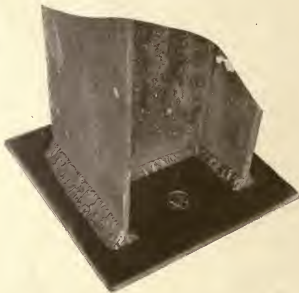
WELDED CONNECTION BETWEEN BASE PLATE AND BETHLEHEM H SECTION COLUMN
