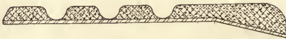
FIG. 16.—TREAD MADE OF ABRASIVE GRAINS IN LEAD MATRIX THE WHOLE CARRIED ON STEEL PLATE, GROOVED TOP
