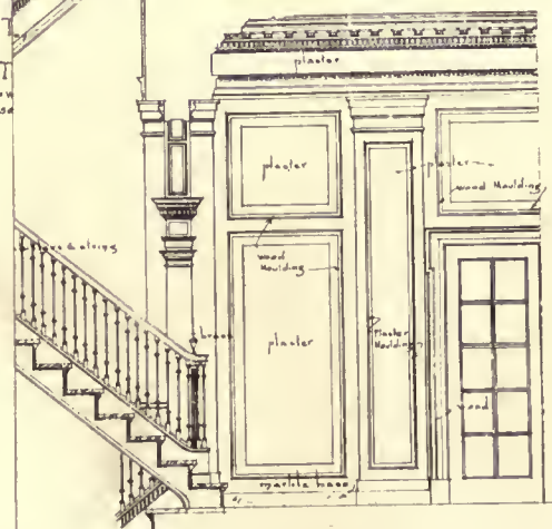
SECTION TYPICAL STAIRCASE
