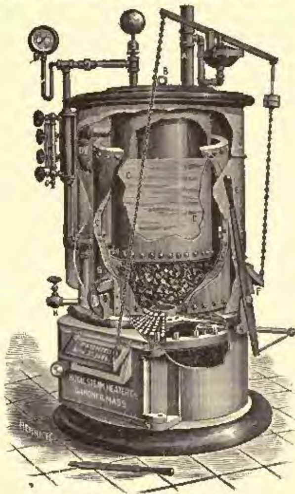
DESCRIPTION OF SECTIONAL VIEW. A—Main Steam-pipe, B—Magazine Cover, C C—Water Spaces, D D—Pipe connecting boiler, E—Lever for shaking grate, F—Check-draft, G—Arrangement for dumping grate, H—Blow-off-pipe to empty boiler, also to be connected with water-pipe for filling.
