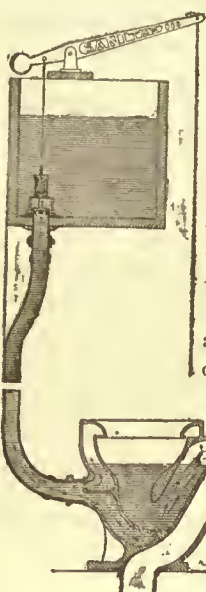
Fig. 35.—Diagram illustrating the Principle of the Sanitas Water-closet.
