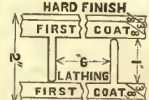
Fig. 7. Section of same, 2 inches thick.
