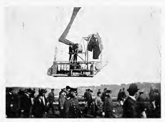
THE CAR OF THE "PARSEVAL" AIRSHIP (Note the collapsible blades of the projeller, and the air fump for filling the hallonet)
