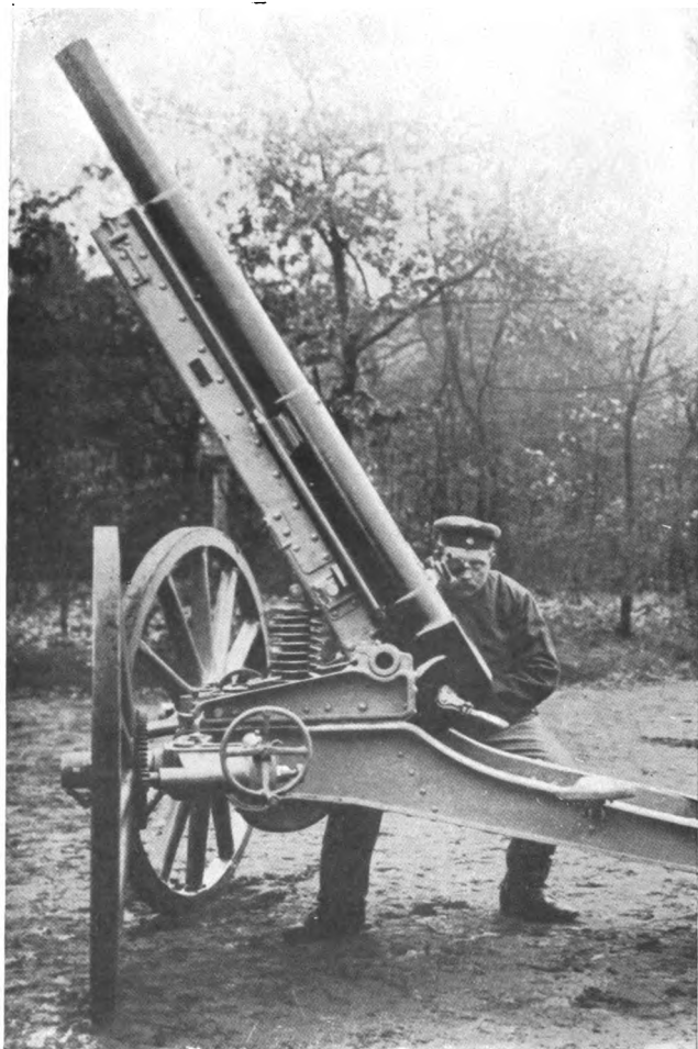
THE LATEST KRUPP ANTI-AIRCRAFT GUN, SHOWING NOVEL DISPOSITION OF WHEELS.
