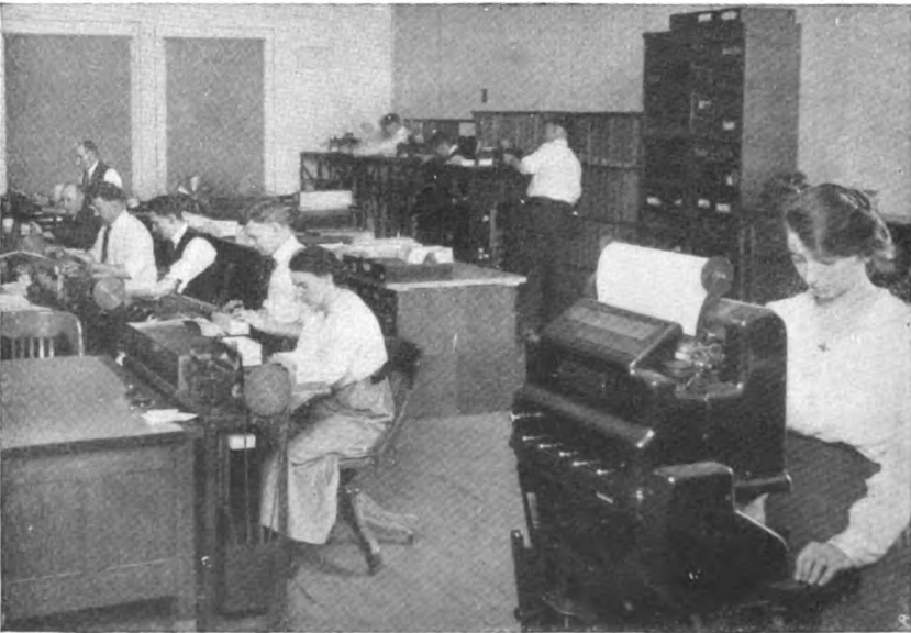
The statistical machine in the foreground handles 250 cards a minute, and an inexperienced girl can easily run it. This is an indication of how much time can be saved by the use of machinery in the bookkeeping department. And time is money.
