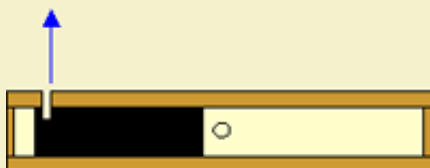
Figure 1: A single action saxon, driven from one end only.
