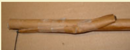
Figure 10: Fusing a double action saxon with piped match.
