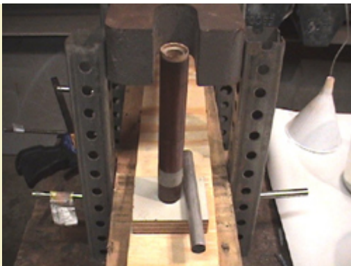
Figure 8: Pressing the 1/2" driver on an arbor press.
