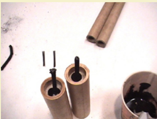
Figure 9: Fusing and priming the drivers.
