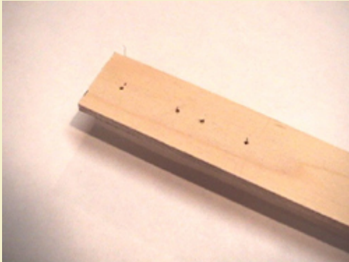
Figure 4: Drilling holes for tie-wires to pass through.
