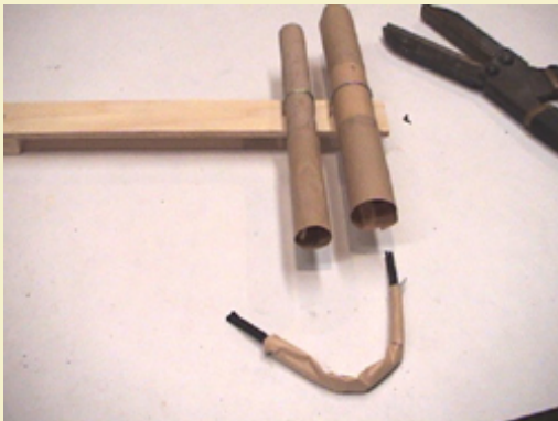
Figure 12: Fusing the drivers so the end of the 3/4" color driver ignites the 1/2" silver driver.
