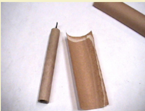
Figure 10: Applying the outer nosing paper.
