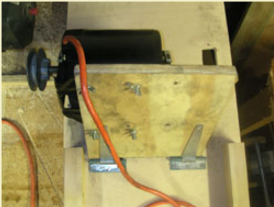
Figure 10: Closeup of motor mounted on hinge plate.
