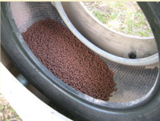
Figure 17: High volume and star uniformity achieved with the tire roller.
