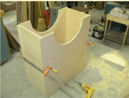
Figure 5: Holding box together with clamps while fitting-out internal components.
