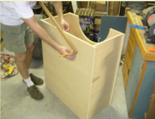
Figure 4: Using a home-made compass to mark the circular cutouts.
