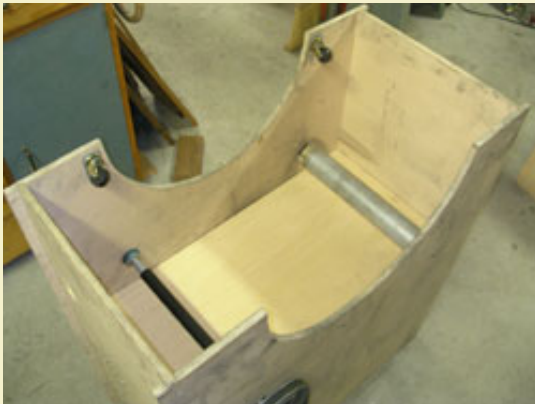
Figure 13: Shelf and rollers installed. Note the swivel casters on each side of the cutout.
