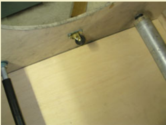
Figure 14: A single central caster is tempting but should be avoided as a potential hazard.
