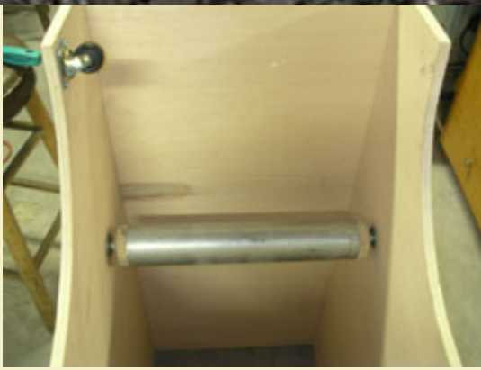
Figure 6: Idler roller installed. Note the castor to prevent the tire from contacting the cabinet.
