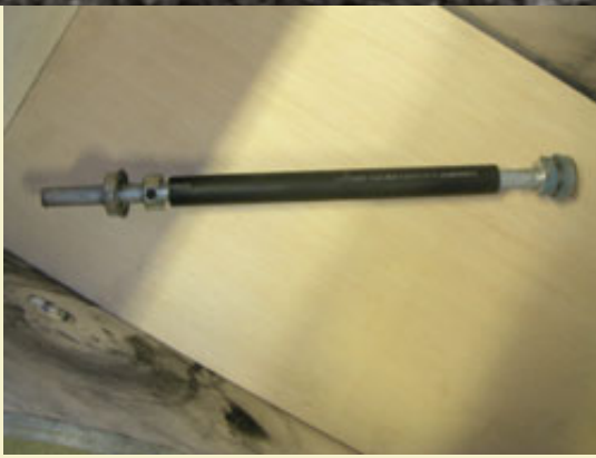
Figure 12: Drive shaft ready for installation after shelf is dropped in place.
