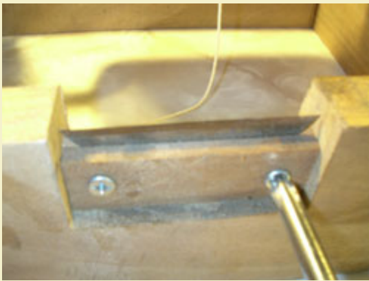
Figure 4: Clamping the blade down by tightening the two wood screws.
