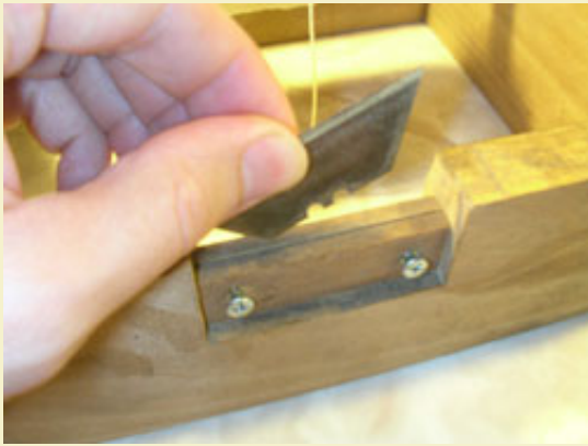
Figure 3: Inserting razor blade between the wood slats.
