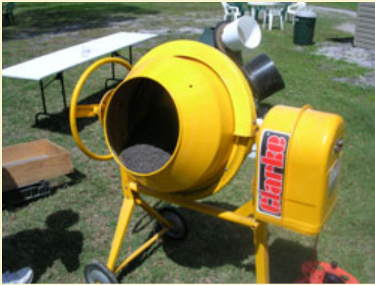
Figure 5: Cement mixers are popular high-volume rollers.
