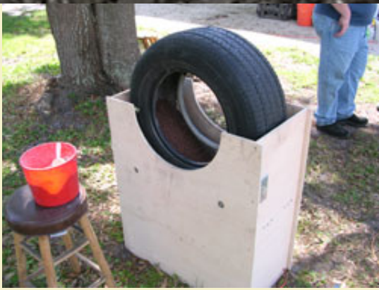
Figure 8: The Passfire star roller using a tire as the rolling drum.
