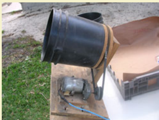
Figure 2: A simple 5 gallon bucket roller.
