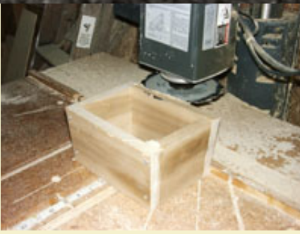
Figure 8: Using a radial arm saw in the horizontal plane to trim top and bottom edges of the box.
