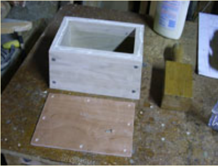
Figure 9: Thin luan plywood is glued flush to the bottom and held by small screws.
