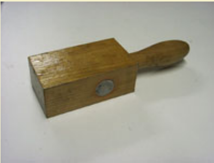
Figure 5: Lead is poured into cavities and hammered flush with sides.
