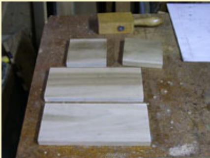
Figure 5: Side pieces prior to cutting side angles.
