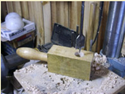
Figure 3: Making holes in rammer to fill with lead.
