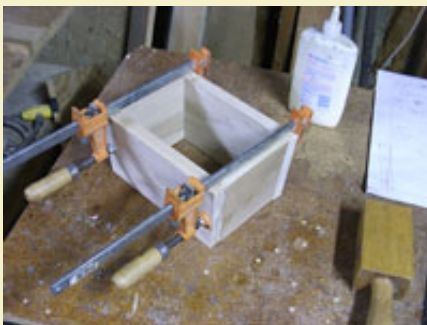
Figure 7: Using bar clamps to glue the pieces together before strengthening with screws.
