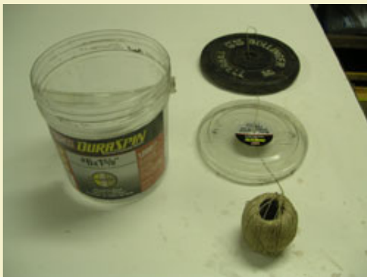
Figure 9: Using a bucket and 10lb dumbbell weight as a string dispensing bin.
