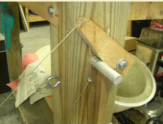
Figure 11: Closeup showing the spiking fixture strung and ready to use. Note the small eyelet to guide the string.
