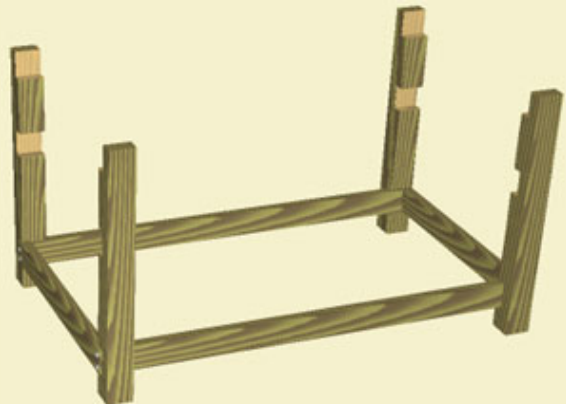
Figure 2: Shelf frames are fastened into notched 4x4 corner posts using one lag screw on each joint.
