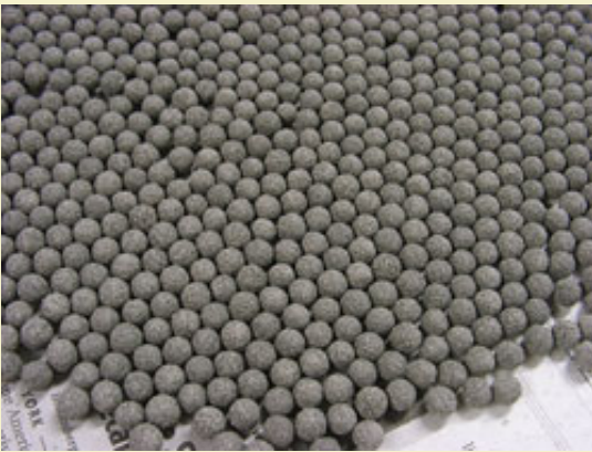
Figure 10: Well sized stars will align into a tight fitting pattern.
