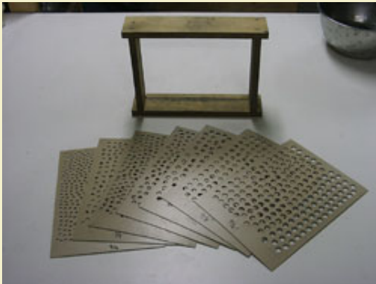
Figure 7: Screen box with interchangeable screens.
