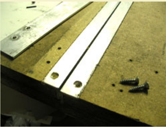
Figure 8: Attaching hold-down bar behind cutting slot.
