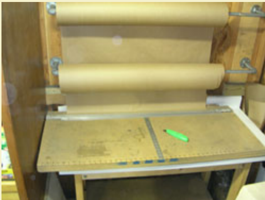
Figure 2: A cutting station that works with both rolls and sheets.
