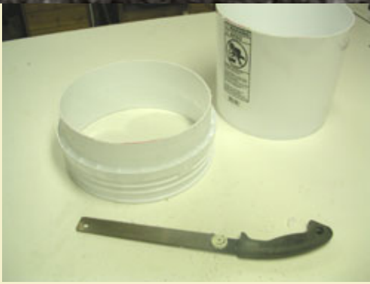
Figure 3: Using a pull saw to cut the bucket in half.
