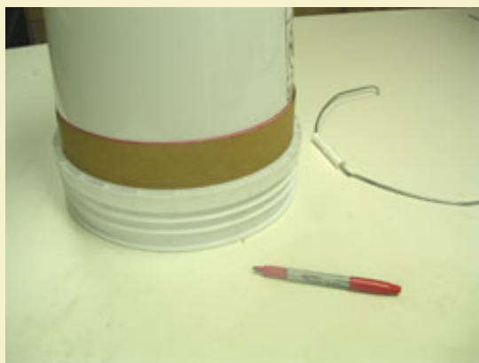
Figure 2: Using a band of paper as a guide when drawing the cutoff line.
