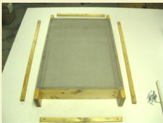
Figure 10: The screen in place (already trimmed).
