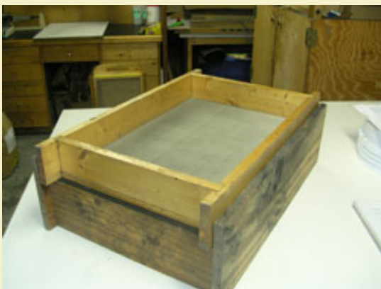
Figure 13: Screen in place atop the mixing box.
