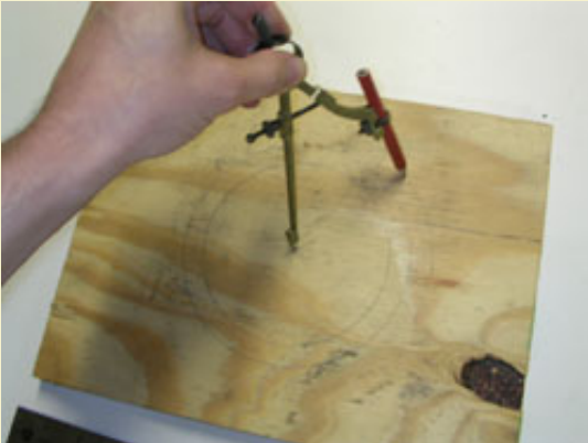
Figure 6: Using a compass to draw concentric disk templates.
