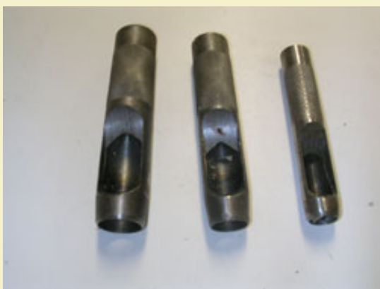
Figure 10: A set of one piece punches with fluted sides for disk removal.
