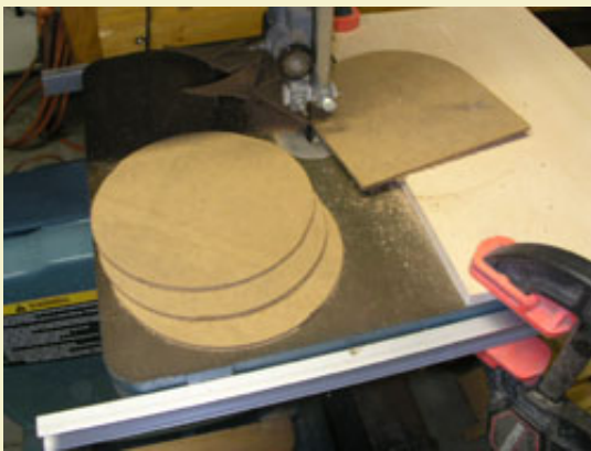
Figure 5: Cutting the circles by rotating the square blanks into the blade.
