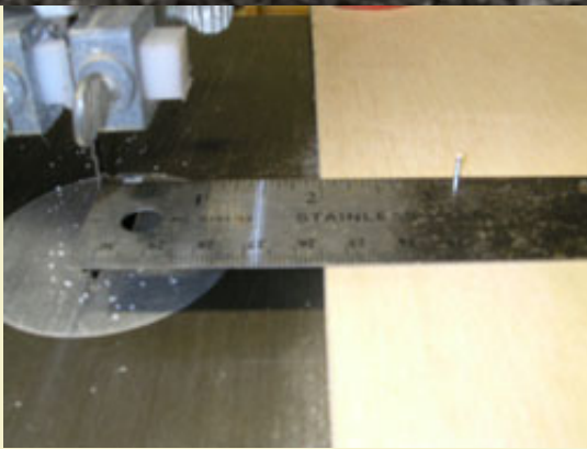
Figure 3: Setting the pin distance equal to the desired disk radius.
