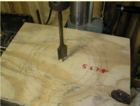
Figure 7: Centering the disk template guide under the bit of a drill press.
