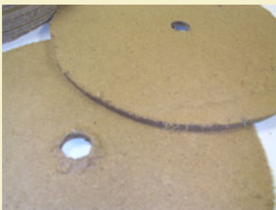
Figure 11: The deformed back-side of a punched hardboard disk compared with a drilled out disk.
