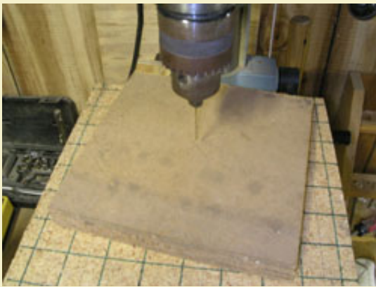
Figure 4: Drilling the center hole through a stack of disk blanks.
