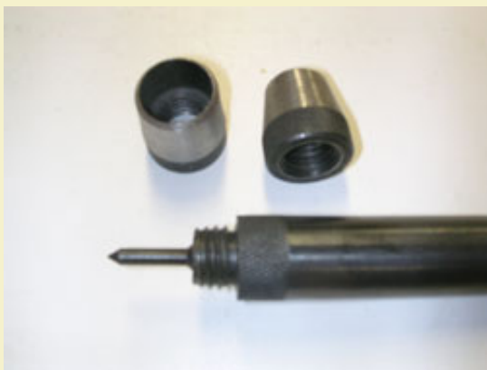
Figure 9: A hollow punch with spring loaded center pin to eject punched disks.
