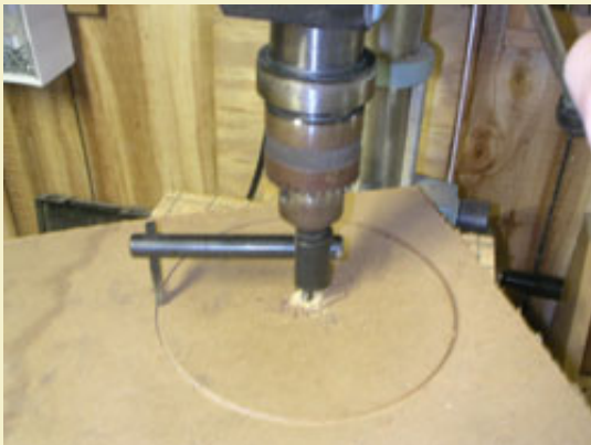
Figure 1: Cutting disks with an adjustable circle cutter.
