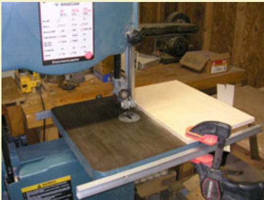
Figure 2: A center pin circle cutting jig clamped to a band saw table.
