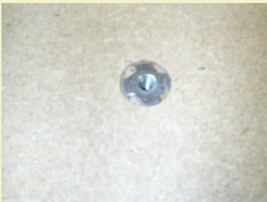
Figure 2: T-nut counter sunk into the center of the bottom disk.
