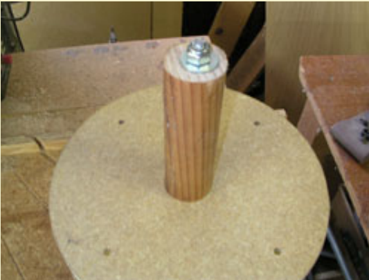
Figure 4: Washer and lock nut fastened at end of handle.
