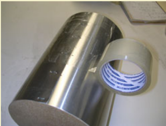
Figure 8: Final protective clear-coat using packing tape.
