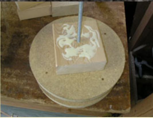
Figure 3: Threading pieces onto the center tie-rod.
