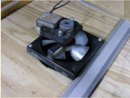
Figure 10: Small fan circulates air through the chambers.
