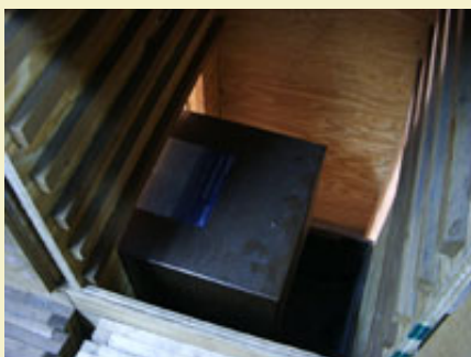
Figure 8: Right side contains dehumidifier to keep air dry.
