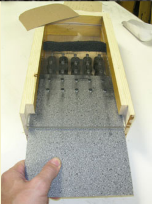
Figure 23: Pulling the barrier plate will drop the equally measured charges into the crossette cavities.
