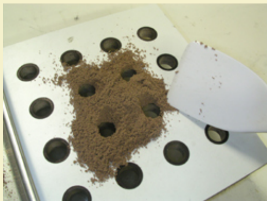
Figure 12: Filling tube array with granulated composition.
