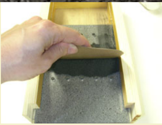
Figure 21: With formica barrier in place, a pile of 2Fg is dragged across the holes to fill them all at once.
