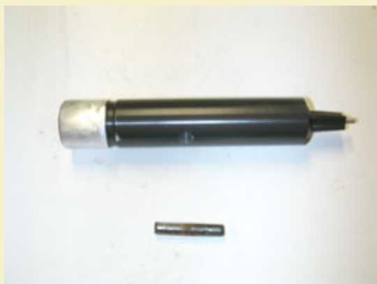
Figure 1: Removing the stop pin from a traditional 3/4" crossette pump.
