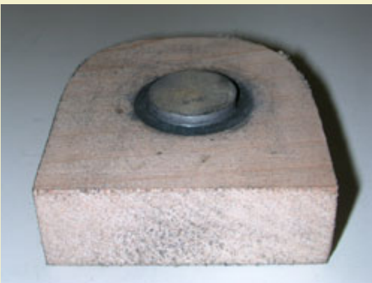
Figure 8: A small nipple is used at the base of the tubes when pressing.
