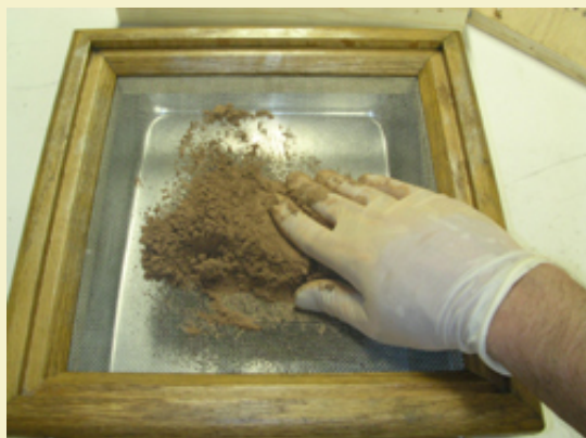
Figure 11: Granulating damp composition through a window screen.
