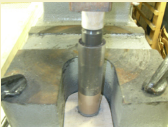
Figure 15: Pressing a crosssette in the arbor press.
