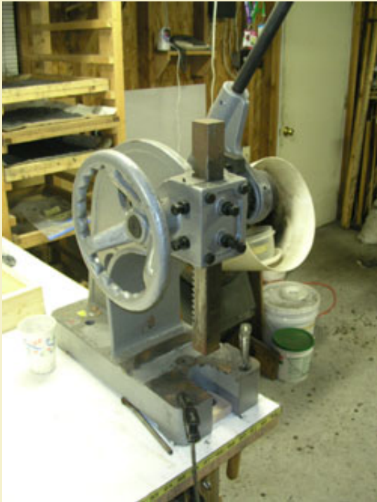
Figure 10: A ratchet type arbor press for easy pulling action.
