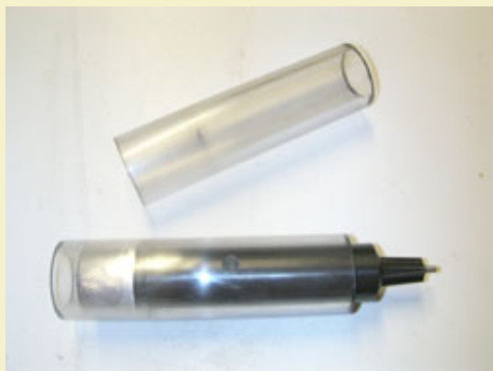
Figure 2: Knurled end is sanded down so that it slides easily through a 3/4" I.D. tube.
