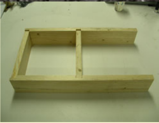
Figure 6: An open ended frame to support the board while loading composition.
