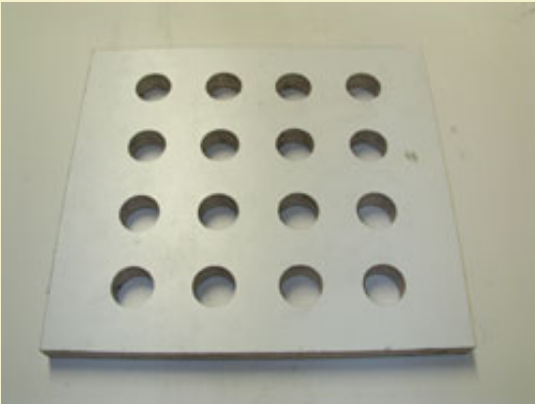
Figure 4: A four by four array of 1" dia. holes drilled in a piece of plastic coated shelving board.
