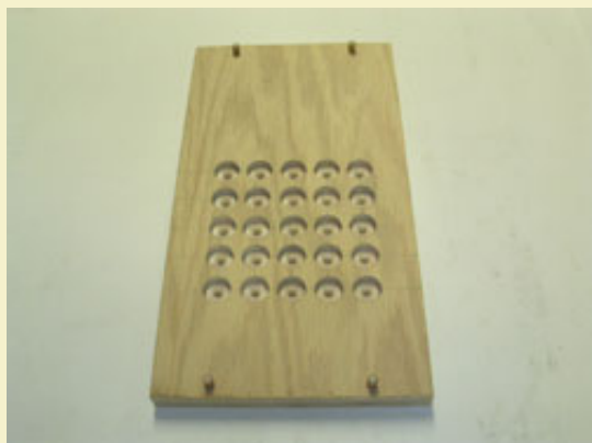
Figure 16: A five by five array of holes drilled 1/4" deep into the base board.
