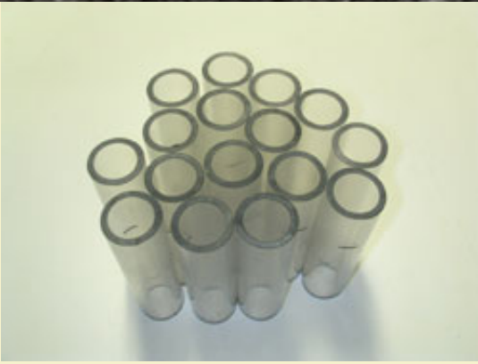
Figure 3: Sixteen polycarbonate tubes are cut to exactly the same height.
