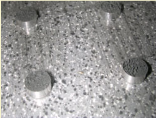
Figure 22: Close-up of 2Fg in the charge holes after scraping away the excess.
