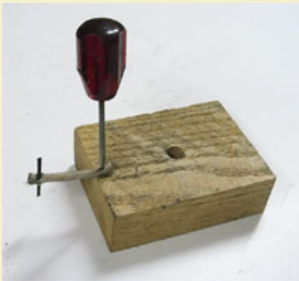
Figure 1: Using an awl to manually punch time fuse.
