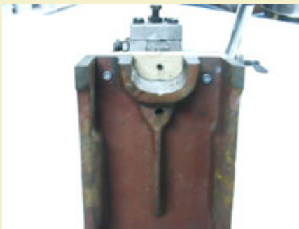
Figure 5: Punch block held to base with two wood screws through the bottom.
