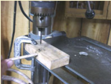
Figure 2: A simple jig that utilizes a drill press as the punching mechanism.
