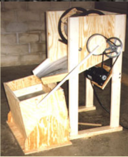
Figure 17: Variation using rocking screen stack to sort grains while corning.
