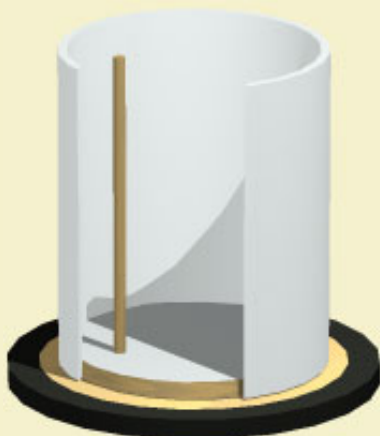
Figure 5: Single 1/2" lift bar located 2" from
