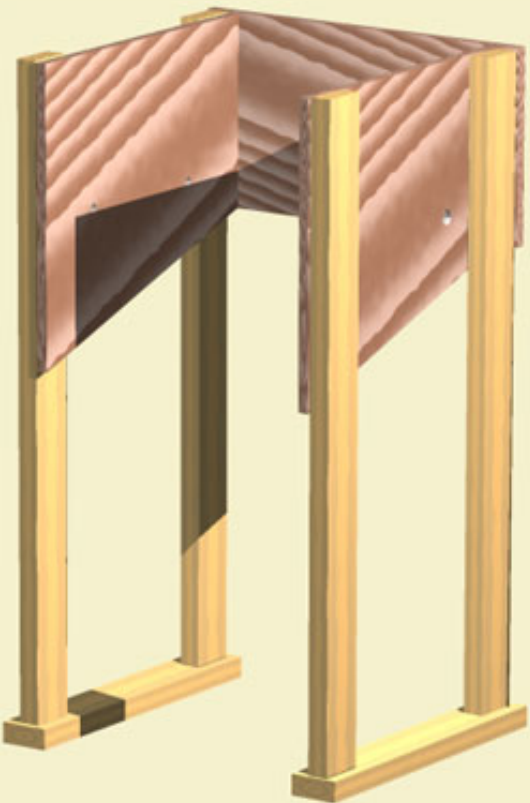
Figure 13: Side panels fastened together with the back panel.
