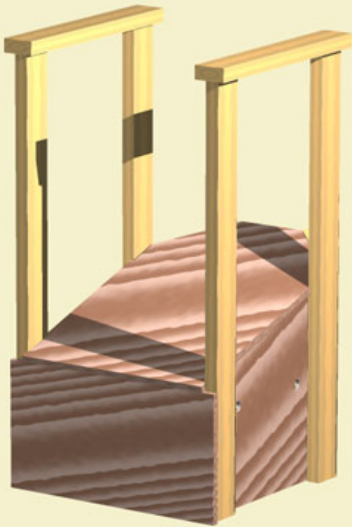
Figure 14: Inverting the corning stand to fasten the bottom panel.
