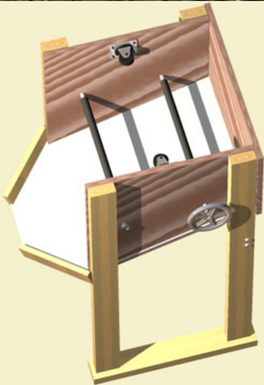
Figure 15: Installing roller bars and casters.
