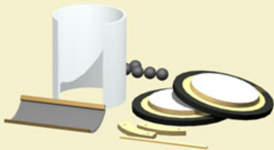
Figure 4: Components for building the corning drum.
