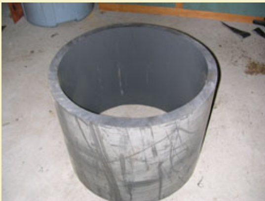
Figure 11: 16" diameter PVC with 1" thick walls for ideal corning drum.
