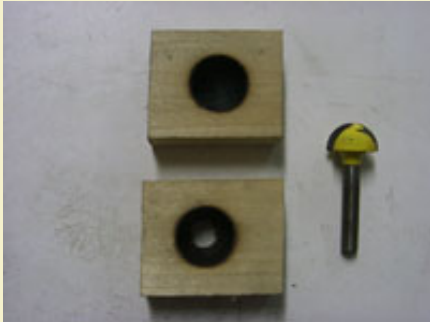
Figure 12: Rounded molds made with a plunge router and a 3/4" half round bit.
