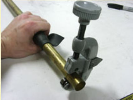
Figure 5: Cutting 1" segments from a long brass tube.
