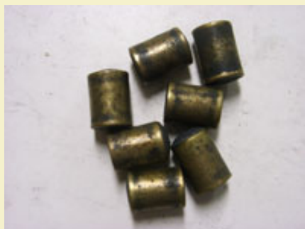
Figure 2: Lead filled brass after substantial usage.
