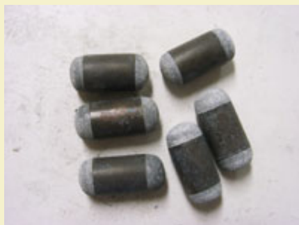
Figure 3: Lead filled brass with rounded ends.
