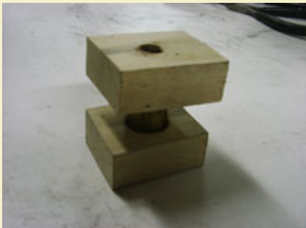
Figure 13: Capping both ends of a brass tube with the half round mold blocks.
