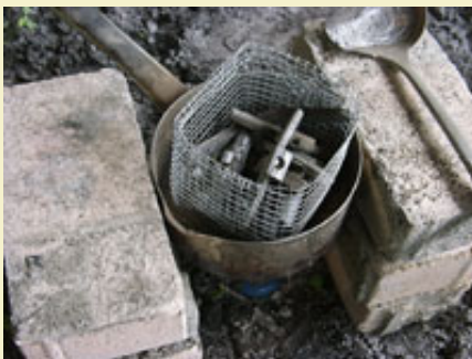
Figure 10: Using a cage to extract metal tabs from tire weights after melting them.
