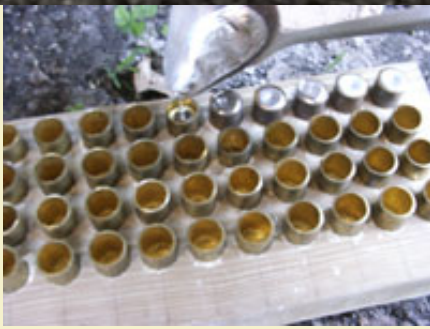
Figure 11: Using the ladle to pour each tube.
