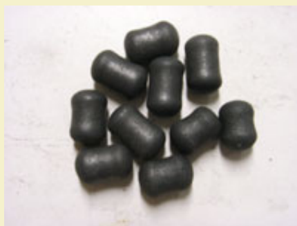
Figure 1: Lead media after substantial usage.
