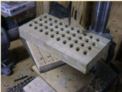
Figure 7: Drilling out the tube holding fixture.
