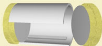
Figure 2: PVC jar with flush fitting ends.
