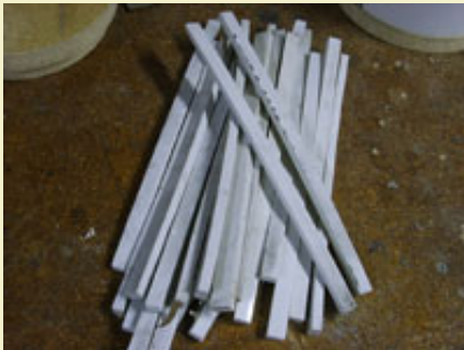
Figure 12: Lift bar strips cut from a section of the PVC pipe.
