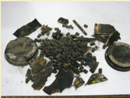
Figure 21: The fragmented remains of the ball mill jar after detonation.
