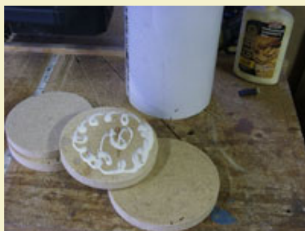
Figure 8: Gluing inner and outer disks together.
