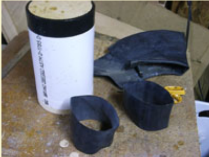
Figure 16: Rubber seals cut from an inner tube.
