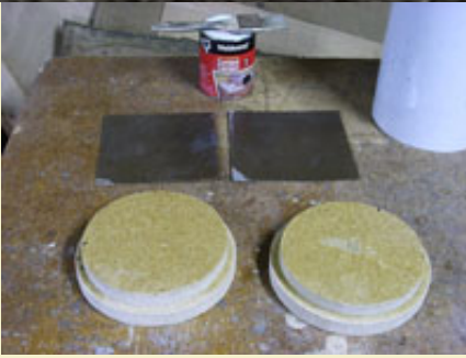
Figure 10: Applying contact cement to disks and Formica scraps.
