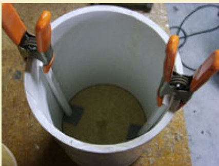
Figure 13 Gluing lift bars into place.
