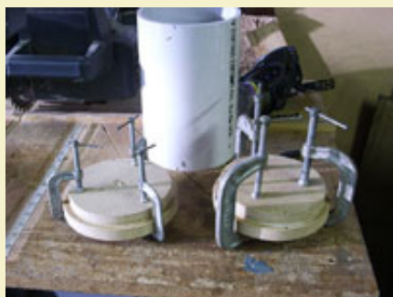
Figure 9: C-clamps used to laminate disks together.
