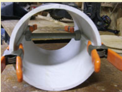
Figure 14: Using a threaded rod with two nuts to hold lift bars flat.
