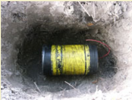
Figure 20: Simulating a mill explosion with a live jar.
