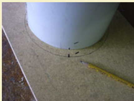
Figure 7: Tracing PVC ends onto particle board.
