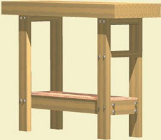
Figure 7: Table with legs framed out for switch box.
