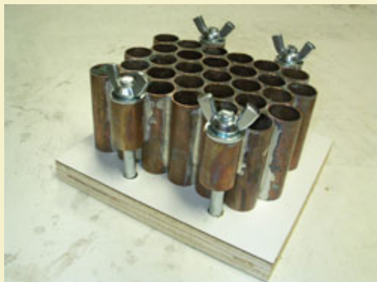
Figure 16: Hole plate fastened to the hold-down plate.
