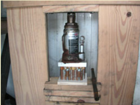
Figure 21: Using the comet plate in a home-made press for creating rock-hard comets.
