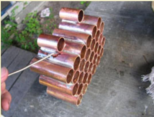
Figure 4: Soldering the shorter clamping tubes to the sides.
