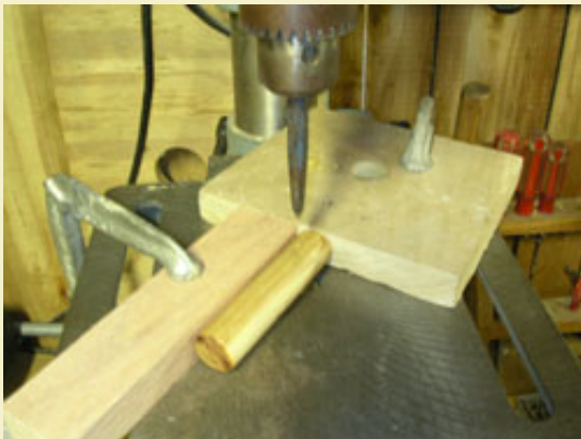
Figure 9: Using a jig to consistently mark the nail position on all pins.
