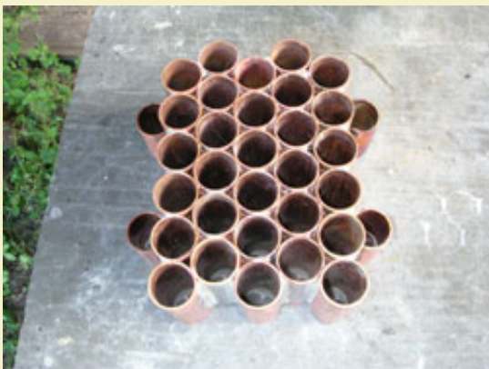
Figure 5: The finished tube block for pumping 30 comets.
