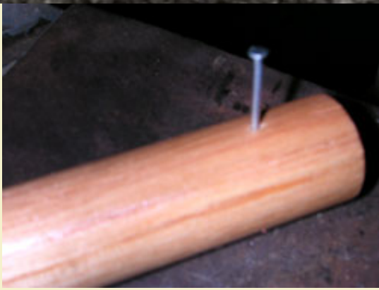
Figure 10: Driving a small nail to be used as a depth stop.
