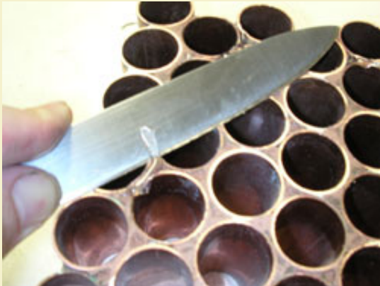
Figure 7: Shaving the solidified glue flush with the surface.
