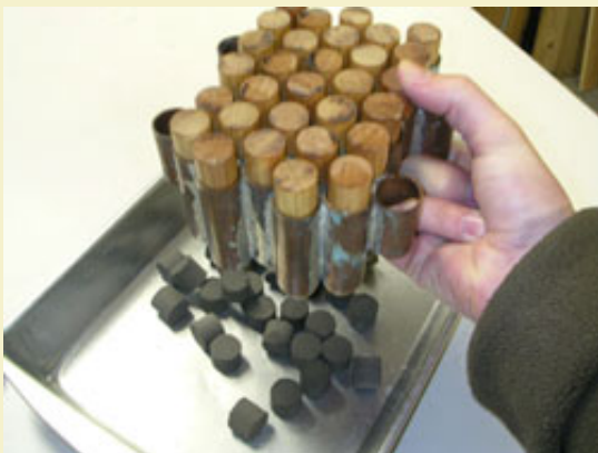
Figure 19: Individual pins allow comets to be pressed out by hand.
