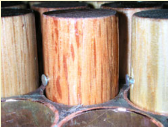
Figure 11: Nail prevents pins from falling all the way through the tube when comets are pressed out.
