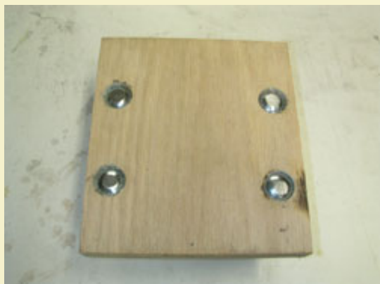
Figure 15: Bolt heads are counter-sunk into bottom of plywood.
