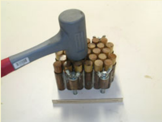
Figure 18: Using a hard rubber mallet to prevent damage to wooden pins.
