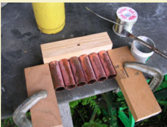
Figure 2: Squaring up a row of tubes to be
