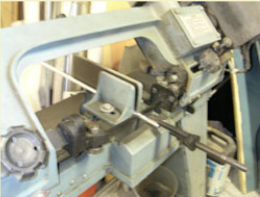
Figure 13: Cutting pins using a horizontal type band saw.
