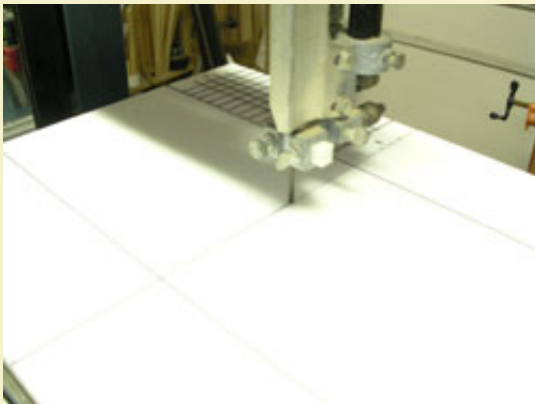
Figure 5: Cutting out the pieces on a band saw.
