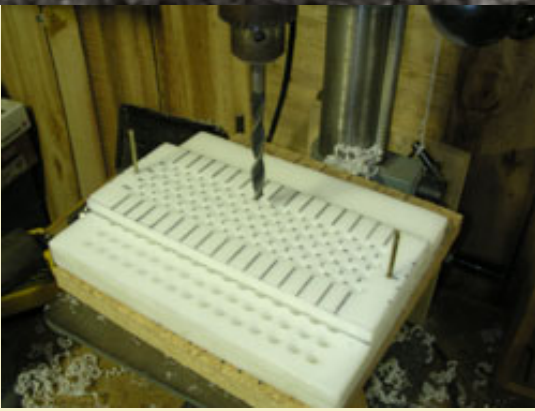
Figure 12: Drilling second group of holes using pin plate as a guide.
