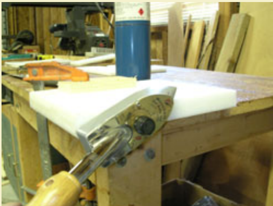
Figure 8: Using a monokote hobby iron to aid in melting the seam together.
