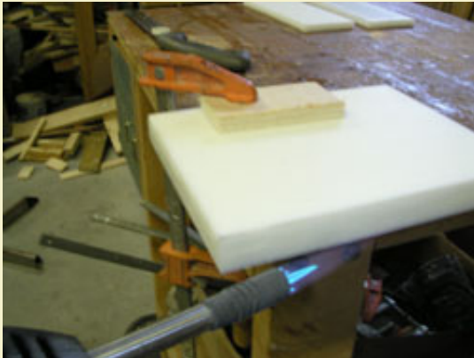
Figure 7: Using a blowtorch to heat the edges when melting the two pieces together into one thick piece.
