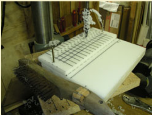
Figure 11: Drilling pin plate and first set of plate holes.
