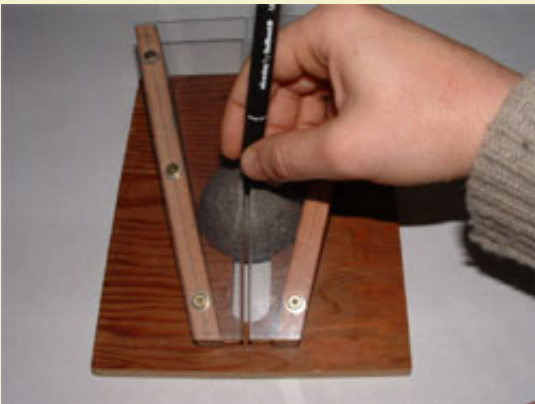
Figure 6: Using the finished center marking jig.
