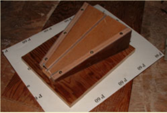
Figure 5: Attaching the two plastic guide sheets.
