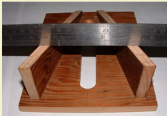
Figure 2: Making sure the top edges are on a level plane.
