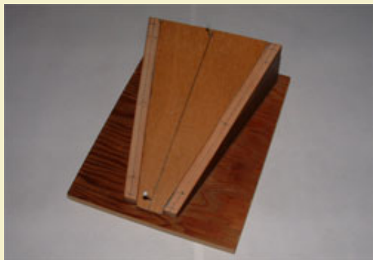
Figure 3: A temporary slot width guide for centering the plastic sheets.
