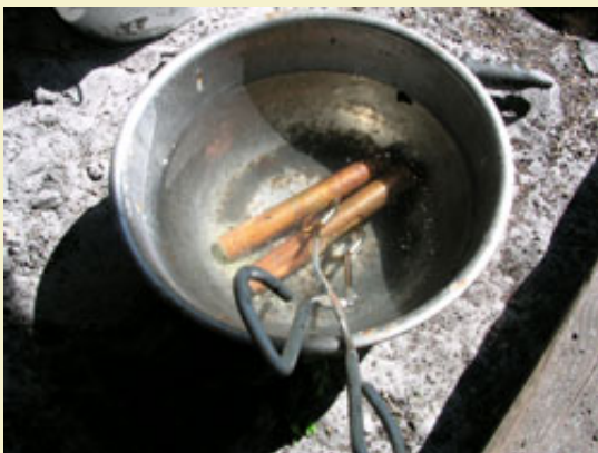
Figure 5: Cooling off the lead in water after it solidifies.
