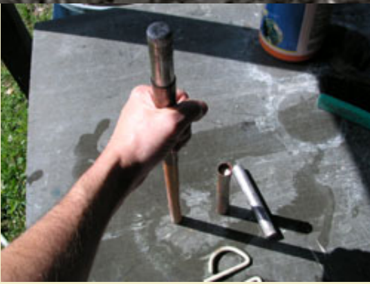
Figure 6: Removing the lead bars from the tubes.
