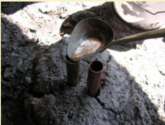
Figure 4: Filling copper pipes buried in the sand.
