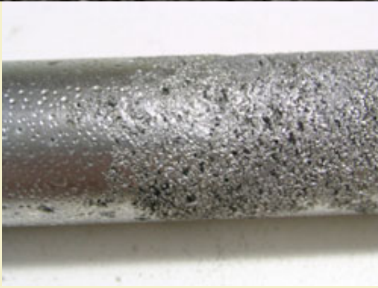
Figure 9: Defect that occurs with certain types of linotype lead.
