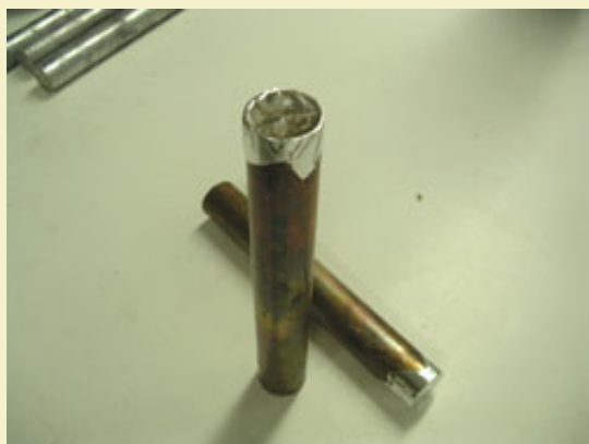
Figure 1: Six inch lengths of copper tubing with foil tape plugging the bottom.
