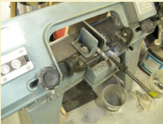
Figure 11: Using a cut-off band saw to make even more rapid cuts.
