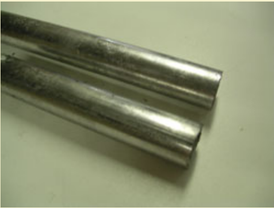
Figure 7: Smooth lead bars ready for segmenting into media.
