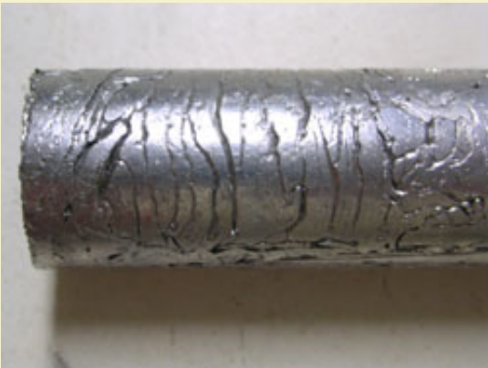
Figure 8: Defect from pouring with lead that isn't hot enough.
