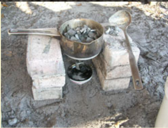
Figure 3: A melting pot made with a Colman propane stove and bricks.
