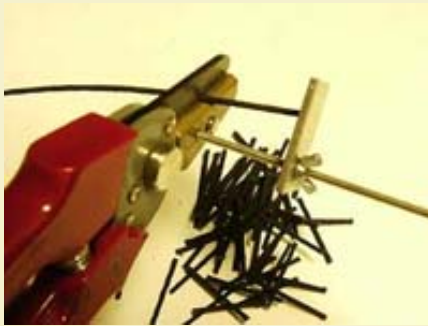
Figure 1: Cutting equal length fuses.
