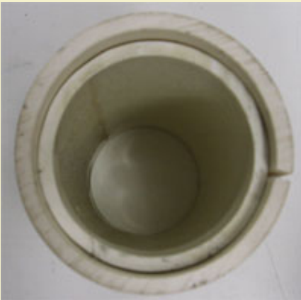
Figure 5: After heating the sleeve should fit snugly over the piston pipe.
