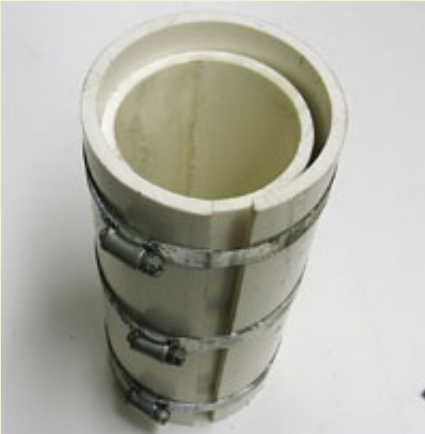
Figure 4: Pipe clamps used to close the gap prior to heating in oven.
