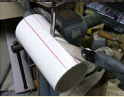
Figure 3: Reducing the diameter of the 4" pipe to 3-1/2" I.D.
