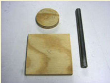
Figure 6: Plywood base, 3-1/2" dia. disk and the 3/4" aluminum rod.
