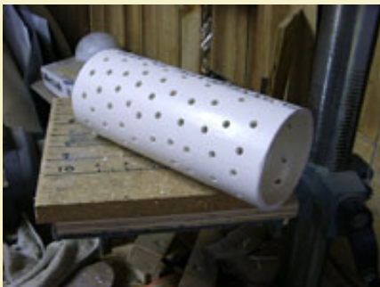
Figure 8: Perforating the piston pipe with 1/4" holes.
