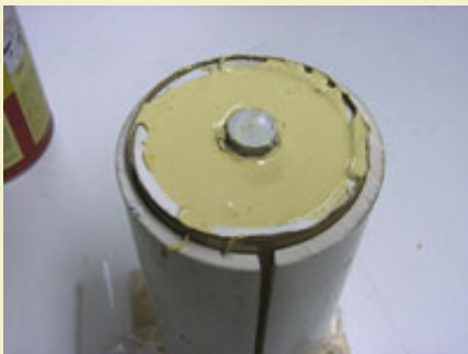
Figure 12: Piston is filled to the top with water putty.
