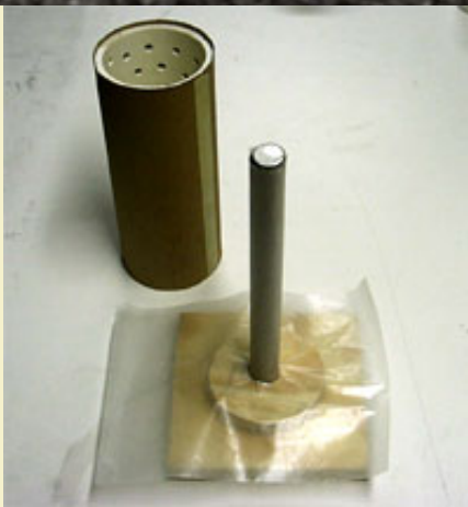
Figure 9: Base and rod are protected with wax paper.
