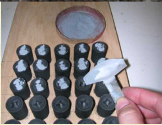
Figure 3: Filling the remainder of the crossette cavity with flash.
