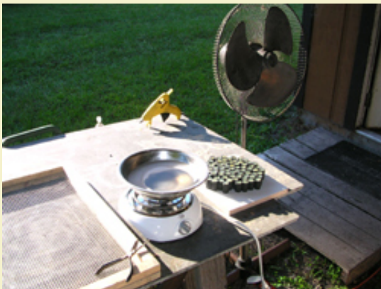
Figure 7: Dipping station includes wax pot, fan and screen.
