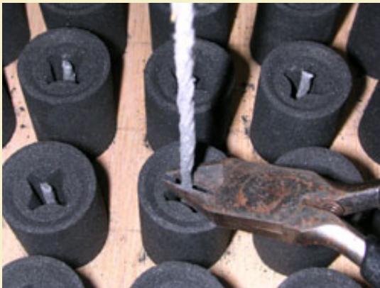
Figure 1: Inserting Chinese paper fuses into the crossette cavity ignition hole.
