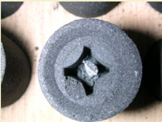
Figure 2: Crossette cavity filled half way with 2Fg.
