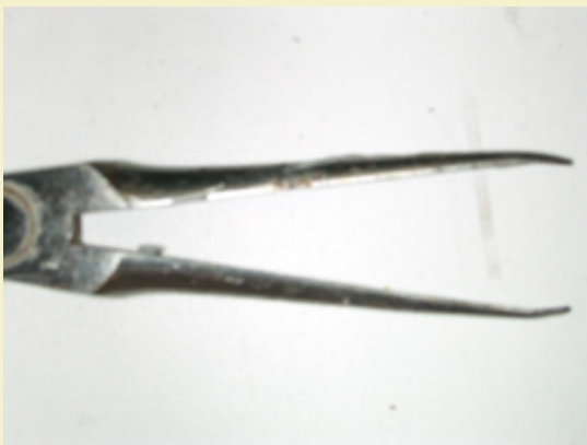
Figure 8: Thin needle nose pliers bent at the tip for holding cassettes while dipping.
