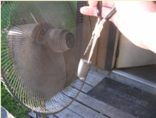
Figure 10: Speed drying the wax in front of a fan.
