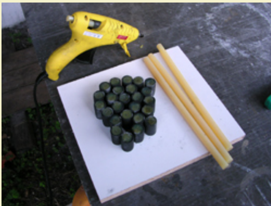
Figure 4: Using hot glue to plug the top of the crossette cavity.
