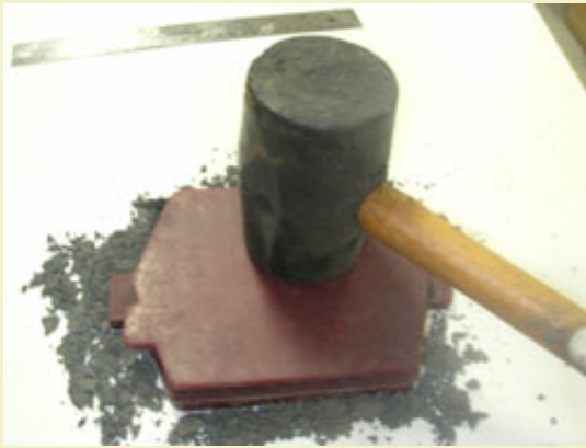
Figure 4: Compacting comp with top plate and rubber mallet.
