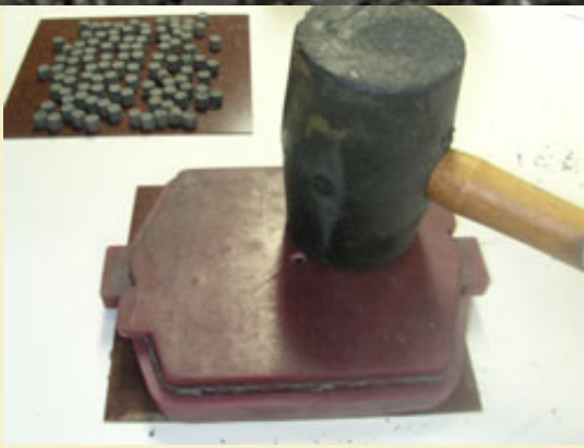
Figure 7: Ejecting stars by tapping with a rubber mallet.
