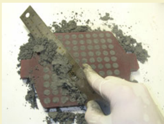
Figure 3: Shaving off excess comp with thin
