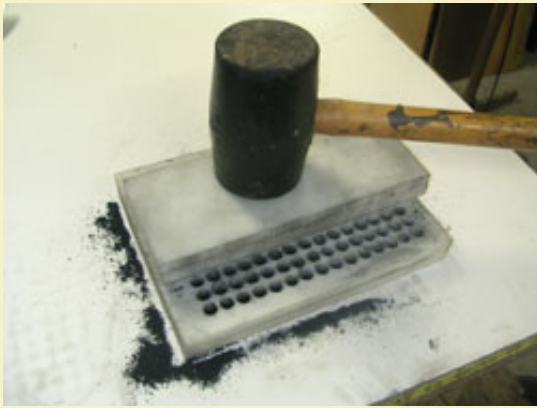
Figure 12: One of three pressings required for this plate.
