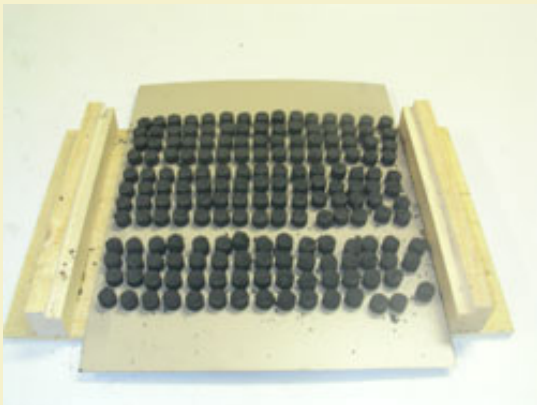
Figure 14: 180 stars ejected onto a removable sheet of plastic.
