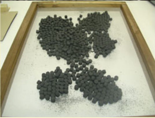
Figure 15: A screen full of pumped stars ready for drying.
