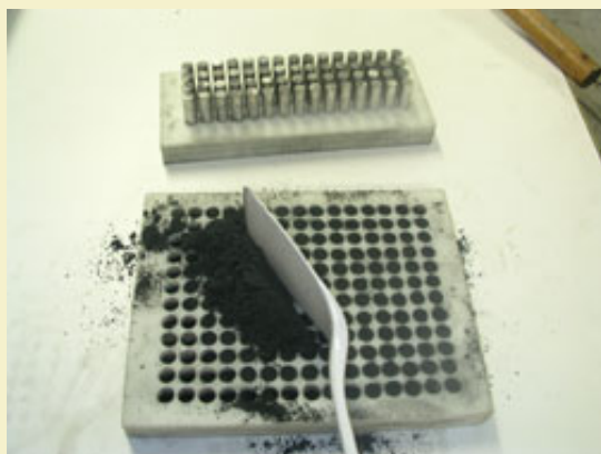
Figure 11: Filling plate holes with granulated comp.
