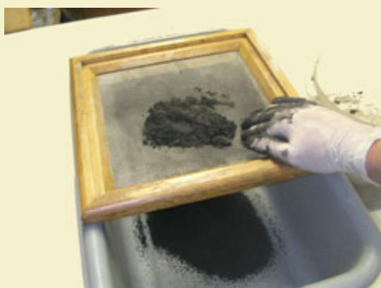
Figure 10: Granulating damp composition through a window screen.
