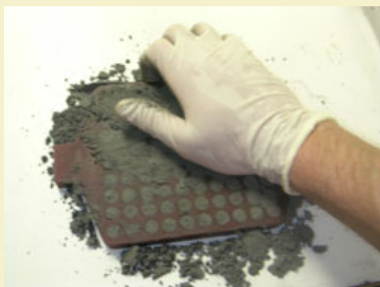
Figure 2: Pushing damp comp into the plate cavities.
