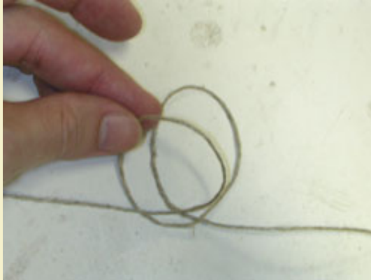
Step 2: The loops are folded together to form the clove hitch pattern.
