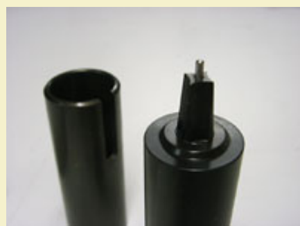
Figure 3: Star shaped cavity former with pin at tip.
