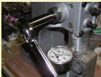
Figure 1: Torque wrench mounted to left side of arbor press shaft.
