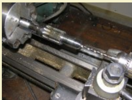
Figure 3: Drill out the shaft to accept a 1/2" tap. In this case, a 27/64" drill was used after a pilot shaft was made with a 1/4" drill.
