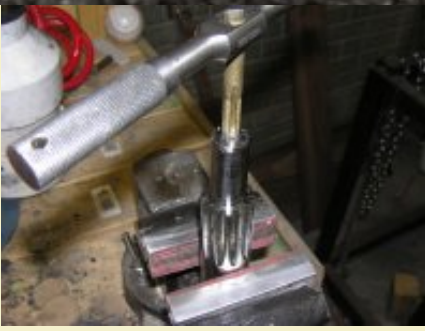
Figure 4: Use a hand tap and carefully cut the threads. If you've never tapped something before, the secrets are to use lubricant, keep things aligned, and go slowly. Cut a quarter turn and back the tap out and repeat. WD-40 will work for a tap lubricant.
