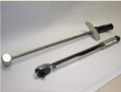
Figure 5: The top torque wrench is the 'beam' type and the bottom wrench is a cheaper micrometer type. The bottom wrench is the most suitable for our project.
