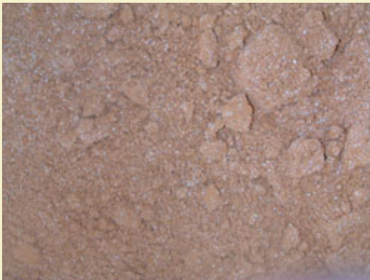
Figure 5: The white specs of stubborn strontium carbonate particles remain after screening is complete.
