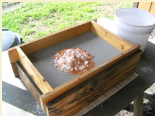
Figure 7: A one pound batch of composition ready to be pushed through the screen.
