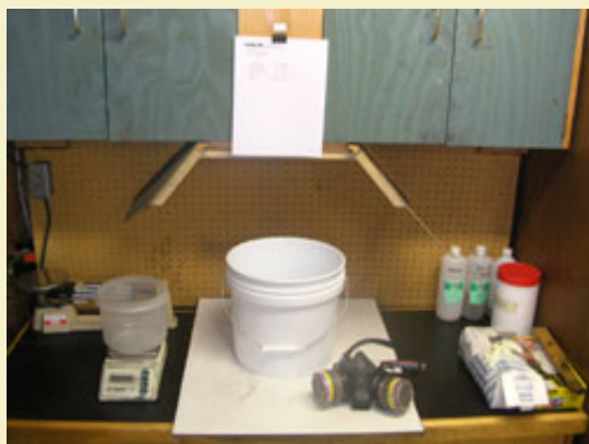
Figure 1: A weighing station for weighing out the components before mixing.
