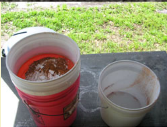
Figure 3: Alternating between two buckets when screening with a bucket screen.
