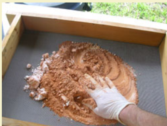
Figure 8: Pushing the chemicals through the screen with a gloved hand.
