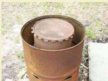
Figure 2: Drum loaded into the furnace.
