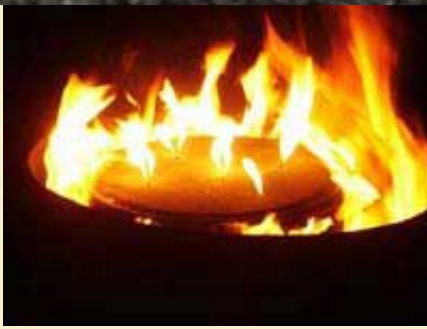
Figure 4: Volatile gases burn bright yellow as they exit the drum.
