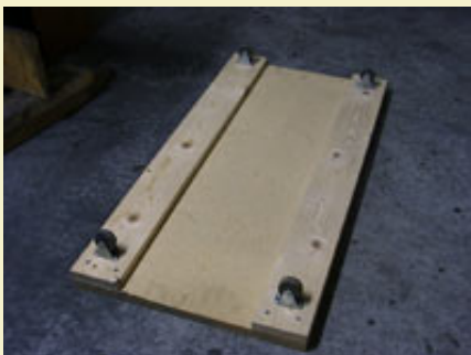
Figure 9: Roller board used to keep the string bucket aligned with the frame.
