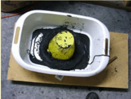
Figure 7: Saturated string placed over a core to prevent entanglement.
