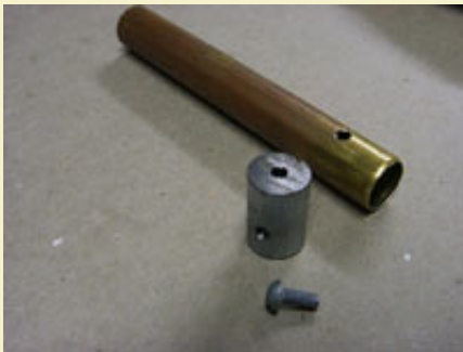
Figure 8: Sizing die used to control diameter of finished match.
