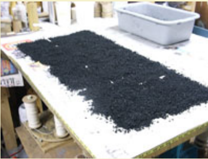
Figure 5: Moving the screen sideways as the chunks are screened results in a thin layer that dries faster.
