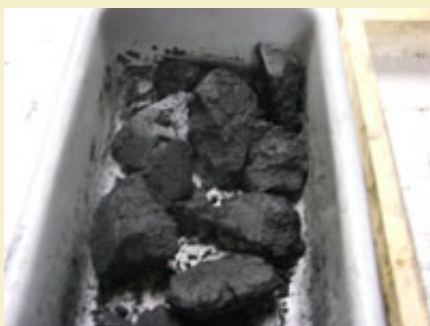
Figure 2: 14% water by weight is incorporated into the powder and formed into big chunks.
