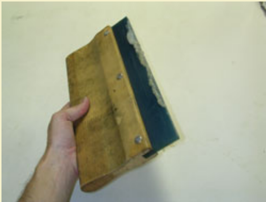
Figure 7: Using a squeegee to quickly clean up the mess from pasting operations.
