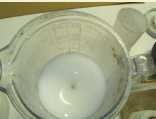
Figure 5: Using the vortex size as a gauge for when the paste is ready.
