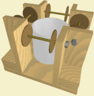
Figure 4: Spools mounted in brackets.
