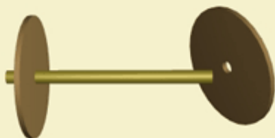
Figure 3: Making spools with brass tubing and 3" end disks.
