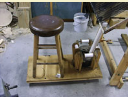
Figure 12: Match making station with slurry bucket loaded and PVC threaded.
