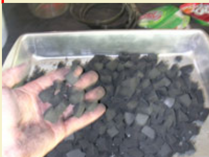
Figure 11: Rough breaking the pucks by hand to feed the corning machine.
