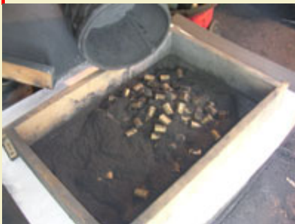
Figure 4: Screening media from meal powder.
