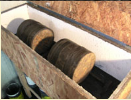
Figure 3: Milling with dual 8" HDPE jars.
