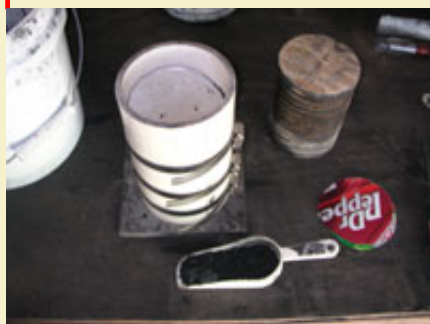
Figure 7: Loading the powder die.
