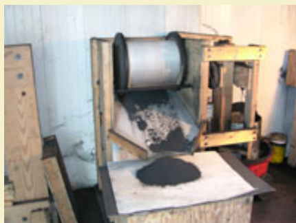
Figure 12: Corning machine in action.
