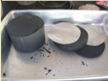
Figure 9: Splitting the pucks apart.
