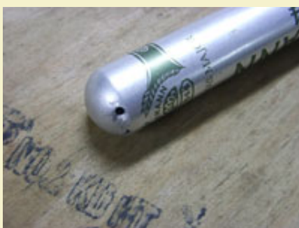
Figure 2: A 5/64" hole drilled at the bottom of a cigar case.
