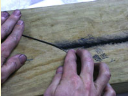
Figure 5: Hand position for rolling up the fuse.
