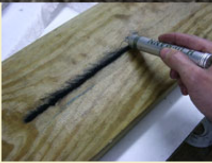
Figure 4: Tapping a powder train with the powder applicator.
