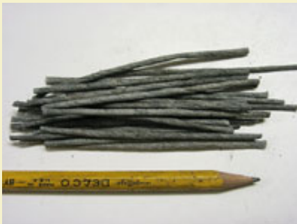
Figure 7: Finished batch of 3/32" diameter fuse.
