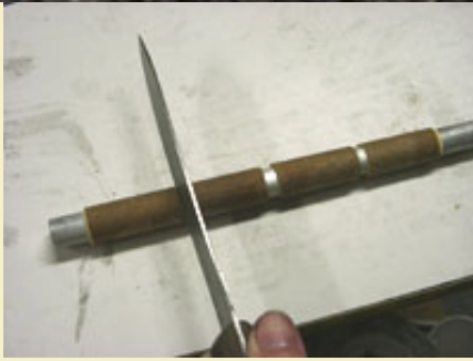
Figure 3: Cutting 6" tubes into 1-1/2" segments.
