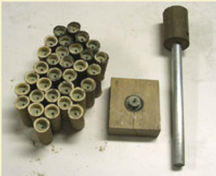
Figure 4: Clay plugs rammed and drilled.
