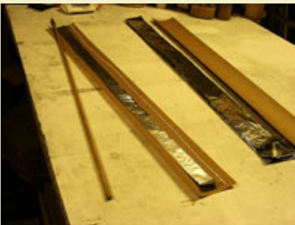
Figure 4: Placement of the foil strip.
