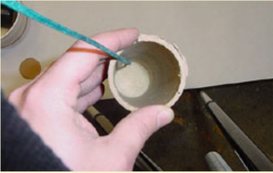
Figure 8: Sawdust is firmly packed around the shell to a thickness of 4" above the lift charge.
