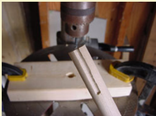
Figure 10: The notched ramming drift.
