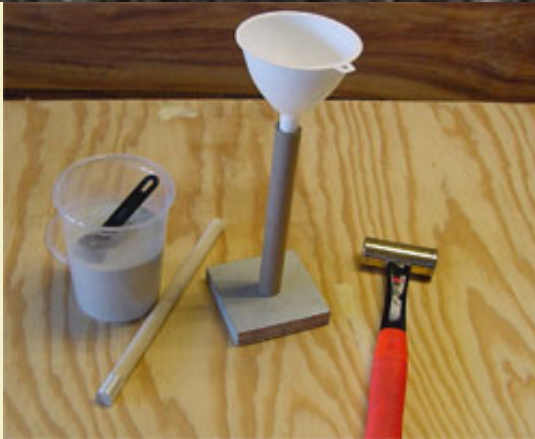
Figure 3: Using a funnel to load the clay bottom plug.
