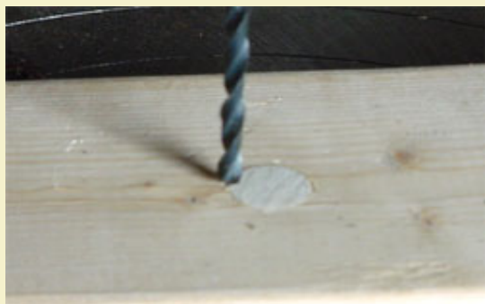
Figure 9: Notching the end of a dowel rod to make the finishing drift.
