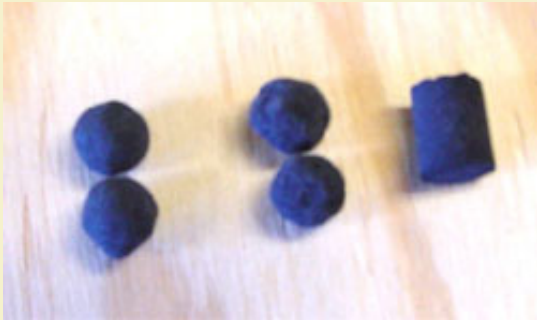
Figure 7: Two types of stars used in roman candles.
