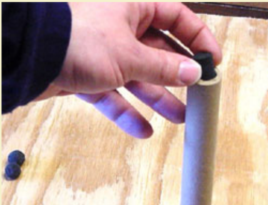
Figure 8: Inserting a star after the lift charge is loaded.
