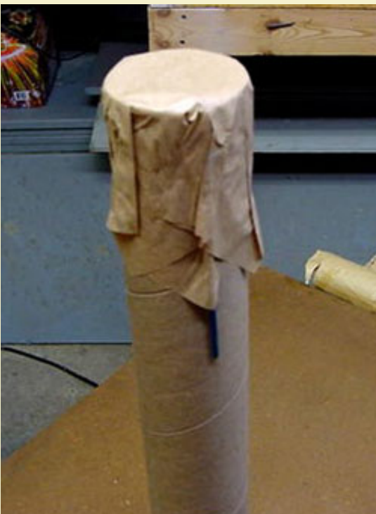
Figure 13: A protective cover pasted over top the candle.
