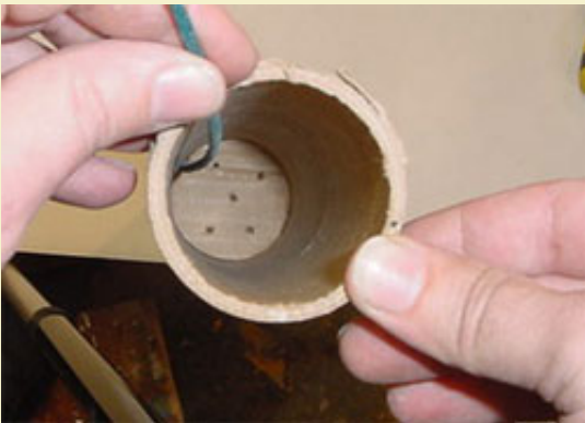
Figure 9: Placing the lift disk over the BP charge on the final mine shot.
