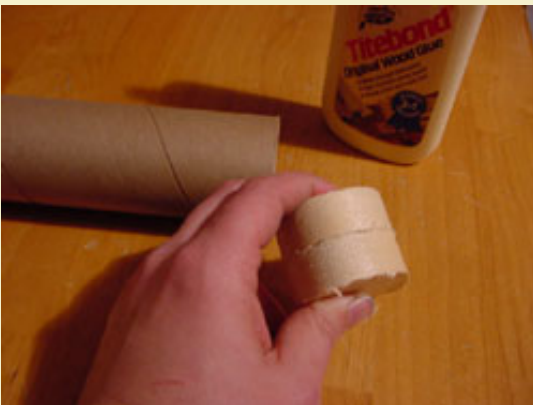
Figure 2: Gluing two 3/4" thick plugs together to form the end plug.
