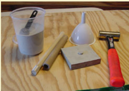
Figure 2: Materials for building a 5/8" candle.
