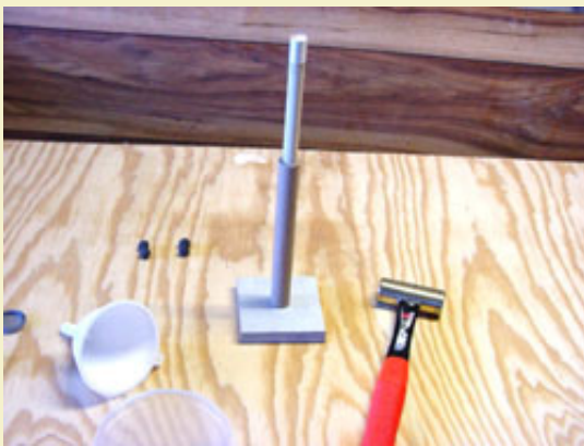
Figure 4: Ramming the clay with a wooden dowel rod.
