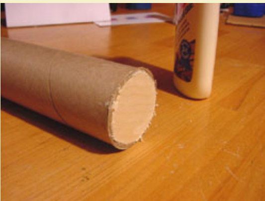
Figure 3: End plug glued in place using wood glue.
