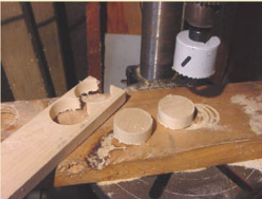
Figure 1: Using a hole saw to cut 2" diameter end plugs.
