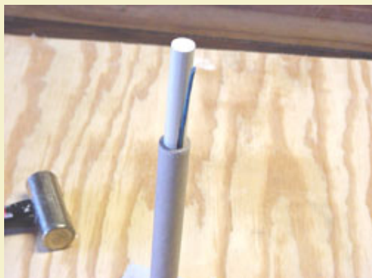
Figure 11: Locking in the fuse with the finishing drift.
