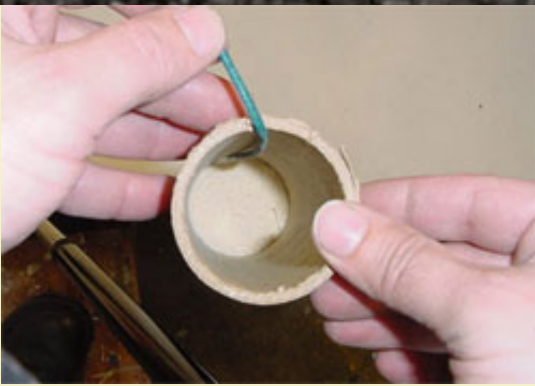
Figure 11: Sawdust packed on top of mine stars.
