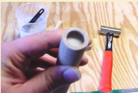
Figure 5: A recessed plug formed from the ramming base.
