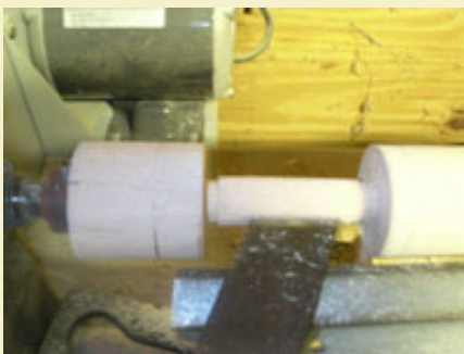
Figure 10: Removing the remaining material with a skew chisel.
