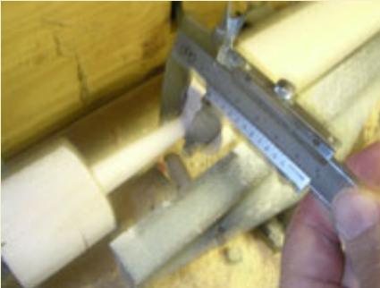
Figure 12: Using a caliper to check critical diameters near the finish point.
