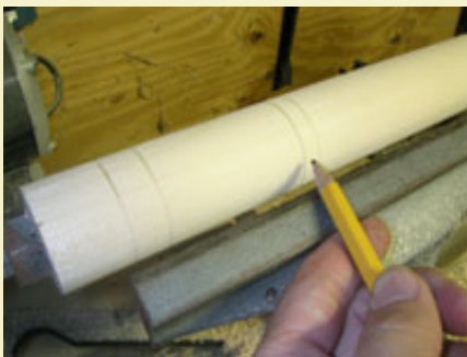
Figure 8: Marking cut points with a pencil while work rotates.
