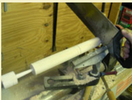
Figure 13: Using a modified hand saw to make three separation joints.
