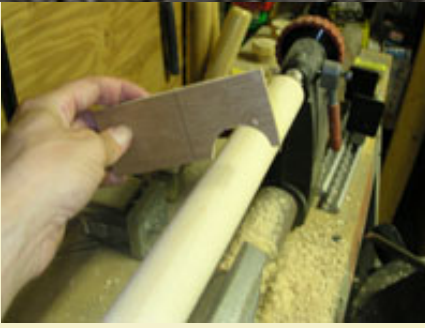
Figure 7: Using a half-circle template to check for proper diameter and evenness.
