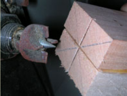
Figure 4: Notching the end to receive the spur center.
