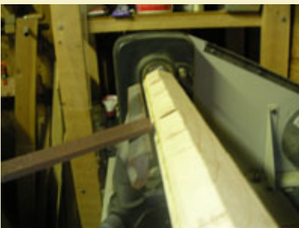
Figure 6: Proper tool rest position.
