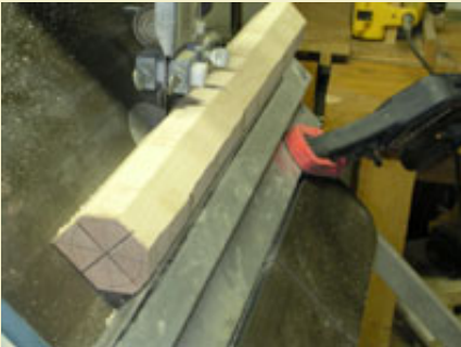
Figure 5: Reducing turning time by shaving off the corners on a bandsaw.
