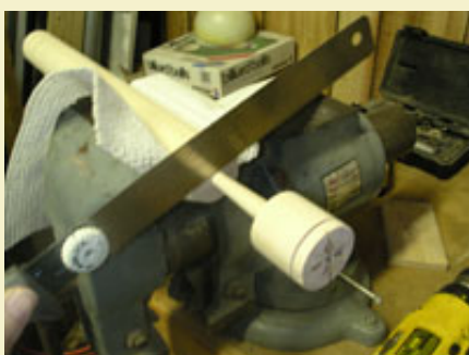
Figure 14: Using a thin kerf pull saw to cut make the final separation cuts.
