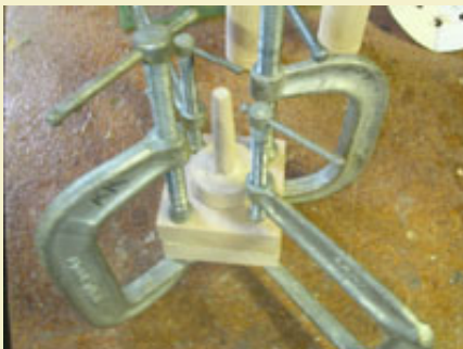
Figure 19: Gluing the spindle and two base plates together.
