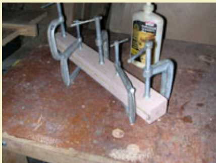
Figure 2: Laminating 1-1/2" thick stock from two pieces of 3/4" thick stock.
