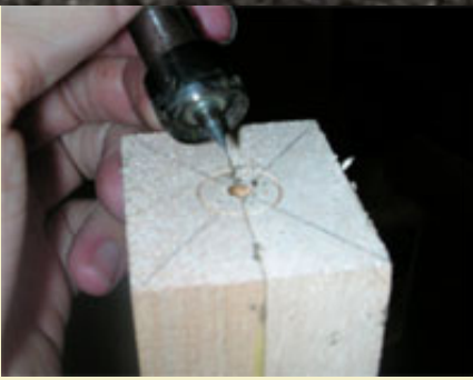
Figure 3: Punching and oiling the tailstock center.
