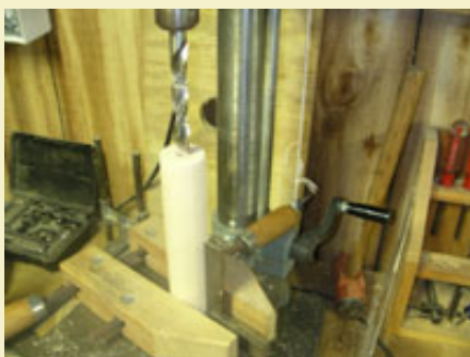
Figure 15: Drilling out the hollow drift with a 1/2" bit.
