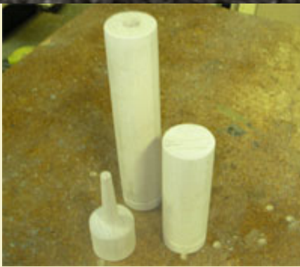
Figure 16: Finished pieces ready for sealing and hardening.
