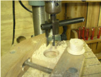
Figure 17: Using an adjustable hole cutter to make a 1.5" hole for the base.
