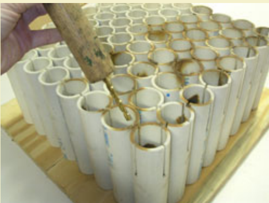
Figure 7: Using a centerpoint guide to mark the hole positions for the bottom plate.
