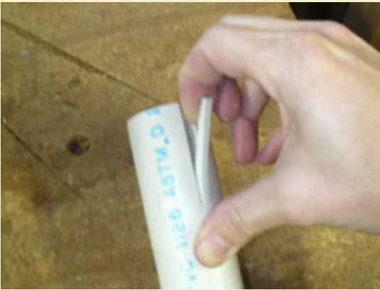
Figure 4: The 1/8" tabs are broken away by hand.
