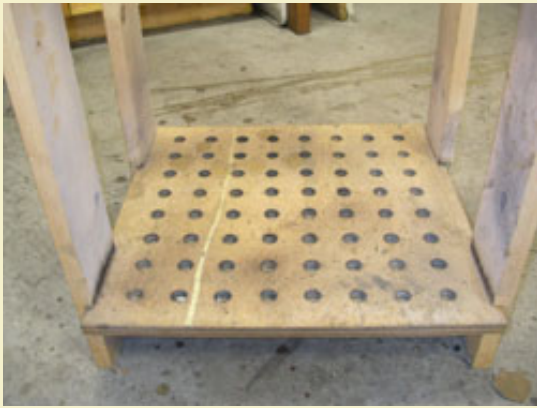
Figure 8: The stick support plate mounted into the leg channels.
