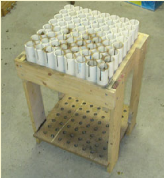
Figure 1: A configurable multi-rocket launch pad.
