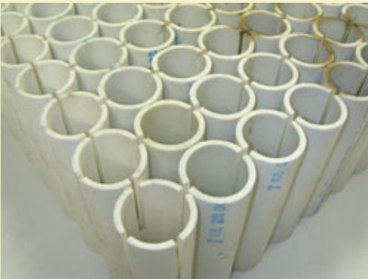
Figure 6: Closeup of passfire slots in finished tube grid.
