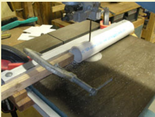
Figure 2: Cutting the passfire slots using a band saw.
